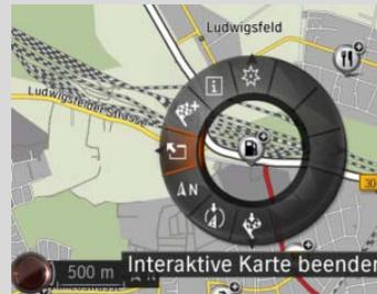
Intelligent routing, addition of **ECO PRO** route and integrated controls via task bars and Pie-menus.
