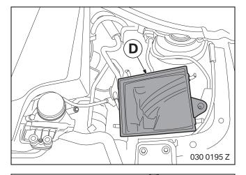
Remove the intake filter housing (see ISTA 13 71 000).
