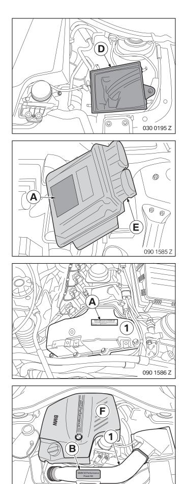
Remove the intake filter housing (see ISTA 13 71 000).
