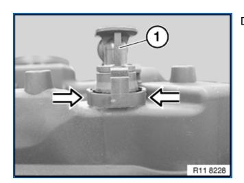
Detach vacuum line (1) in upward direction.
