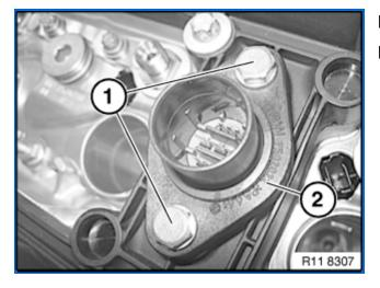
Release screws (1). Remove flange (2).
