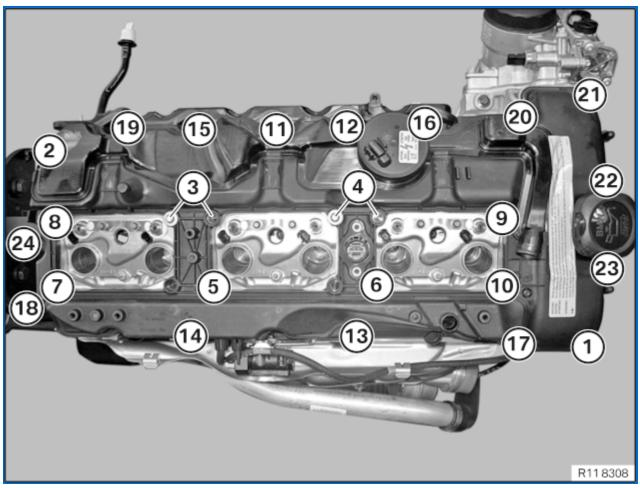
Release screws of cylinder head cover from outside inwards in 1/2 turns.
