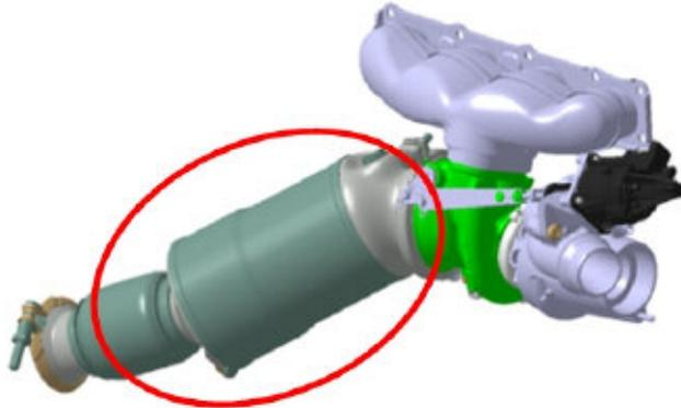
There is an additional catalytic converter located under the vehicle downstream of the exhaust. This converter is not monitored and contains 400 cpsi.
