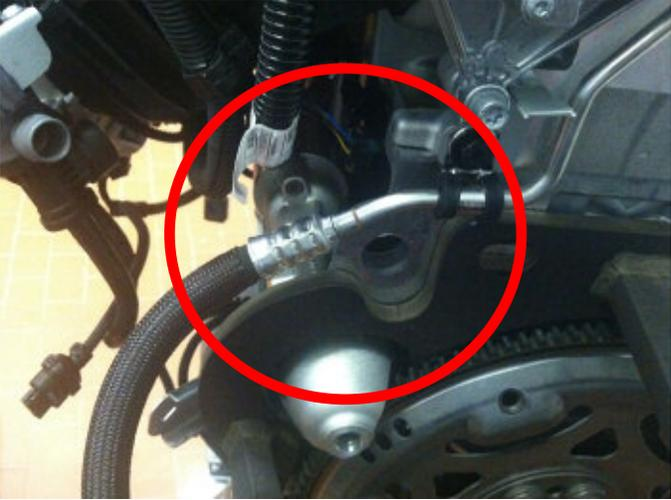
Quick connection on fuel line in engine compartment. This line connects to plastic fuel line to the fuel tank.
