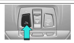
To initiate an emergency request, press the SOS button at the front of cabin roof, then press the button inside the cover.
