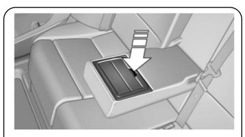
To access the cup holders and armrest, fold down the central console and press the button to open.
