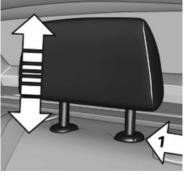
Your headrest can open to an upright position and be adjusted by height. Please fold down headrests before exiting the vehicle.
