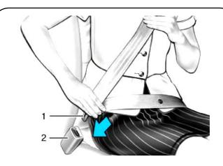
To fasten seat belt, insert tab (1) into buckle (2). Press the red button on buckle to release. Seat belts must be fastened until parking position is reached and vehicle is at full stop.
