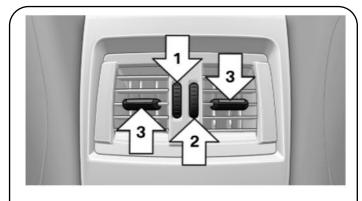
To adjust your climate control, use wheel (1) to control airflow. To vary the temperature, use wheel (2). To direct airflow, move lever (3) to desired position.
