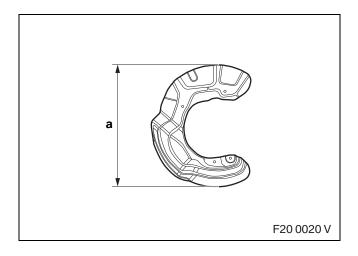
\* Front brake guard plate **H** is only required if 16" brake guard plate with a diameter of **a = 320 mm** is installed.
