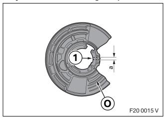
Create two full-thickness cuts in brake guard plate **O** in the centre in the brake calliper cut-out (1) using suitable tools at a distance of **a = approx. 10 mm**.
