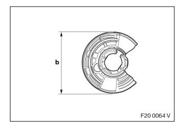
\* Rear brake guard plate **O** is only required if 16" brake guard plate with small wheel bearing and a diameter of **b** = **330** mm is installed.
