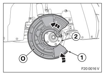
Push the end (1) of brake guard plate **O** from underneath below the driver flange hub (2), then turn brake guard plate **O** to the left.
