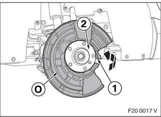
Press the end (1) of brake guard plate **O** over the driver flange hub (2).
