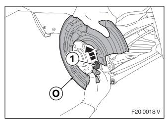
Thread the retaining ring (1) through the hole in brake guard plate **O** and continue to turn it until the retaining ring (1) is fully in front of brake guard plate **O**.
