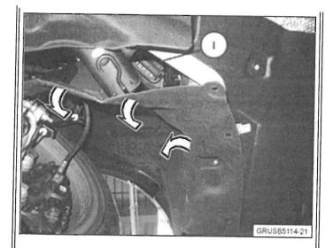
4. Pull the wheel house trim down partially to expose the drain plug. The picture shows the oval E-box drain plug (1) from underneath the vehicle.
