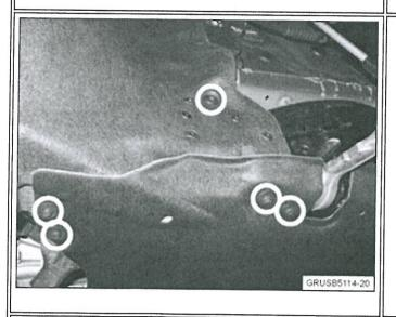
3. Remove the five fasteners as shown.
