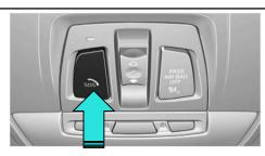
To initiate an emergency request, press the SOS button at front of cabin roof, then press the button inside the cover.
