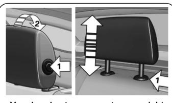
Your headrest can open to an upright position and be adjusted by height. Please fold down headrests before exiting the vehicle.
