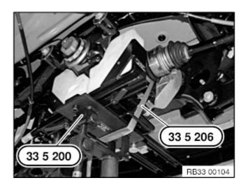
Place the special tool  $\underline{335200}$  onto the universal jack .
