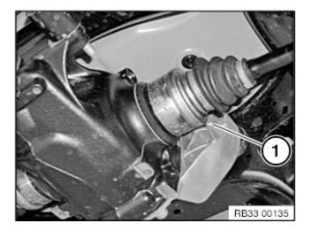
Release nut (1) and push screw towards rear to the limit position.
