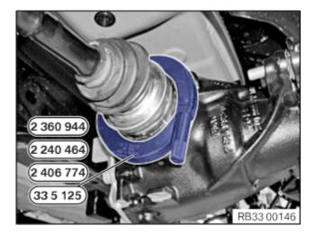
Drive in output shafts into the rear axle differential using the appropriate special tool  $2 \ 360 \ 944$ ,  $2 \ 240 \ 464$ ,  $2 \ 406 \ 774$  or  $33 \ 5 \ 125$  and a rubber mallet. *Installation note:*
